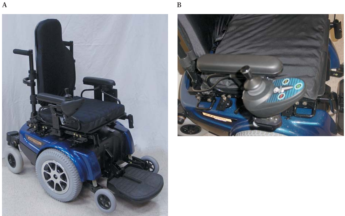
Figure 5.29. A power wheelchair provides a significant amount of independence for children with CP (A). The use of the chair, however, requires specific criteria of cognitive ability, behavioral stability, and motor function. Specifically, the child has to be able to control the chair through some controller mechanism, with a joystick being the most common arrangement (B).
