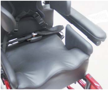
Figure 5.36. There are many different seats available as options for wheelchairs; however, most have some contouring, and many have anterior elevation to place more weight on the fleshy anterior thigh than the bony, more posterior iliac crests and sacral prominences.
