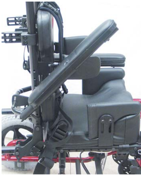
Figure 5.34. Armrests are almost always needed for children with CP because they almost universally need to use the arms to help with trunk balance. If the wheelchair is often pushed up to tables to work, study, or eat, the armrests should be flip-up in nature so they can be brought out of the way of getting under a table surface.
