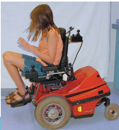
Figure 5.31. The deluxe power wheel base (A) allows power floor sitting (B), standing, seat raising, reclining, tilt-in-space, and foot elevation. These systems are expensive and often require a high level of maintenance.
